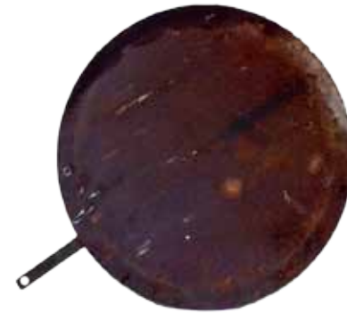
TITLE: Flange Blocker Bung YEAR: 1997 ARTIST: Jim Redgate MATERIAL: Steel DESCRIPTION: Used to block oil pipes at Port Stanvac refinery to pressure test for leaks PRICE: not for sale
